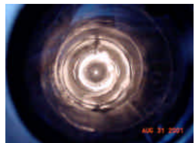
Looking down observation tube with maximum power on in the WESP.
